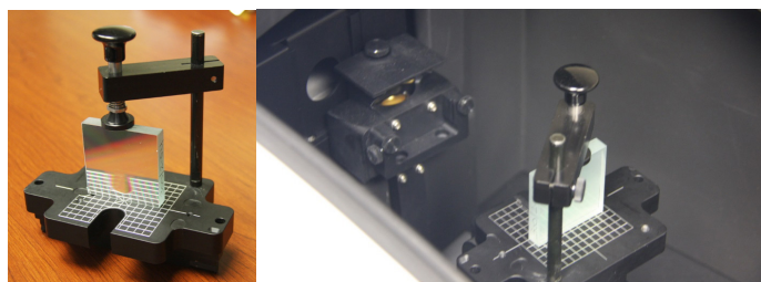
Figure 2. Left: A grating with 300 lines per mm was mounted on a Cube Beam Splitter Sample Holder. Right: The sample holder, placed onto the sample stage in the Cary 7000 UMS. Detector held at 10^{\circ} .
