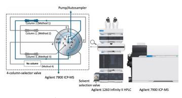
**Figure 1.** Schematic of the HPLC-ICP-MS system with Quick Change valve head used in this study. The 4-column-selector valve head and quaternary pump enabled automated selection of the different HPLC columns and solvents.
