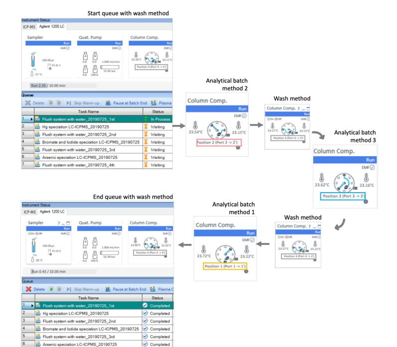
Figure 3. Schematic showing the automated HPLC-ICP-MS procedure controlled by ICP-MS MassHunter software.
