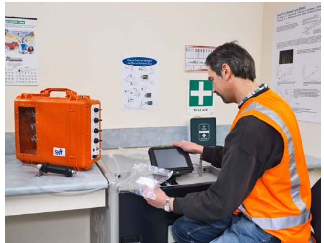
Figure 4. Syft Technologies' Sample Case holds three 1-liter Tedlar or Kynar sample bags, which are removed for Voice200 analysis as shown. The operator uses the integrated touch screen display to start testing and to view results.
