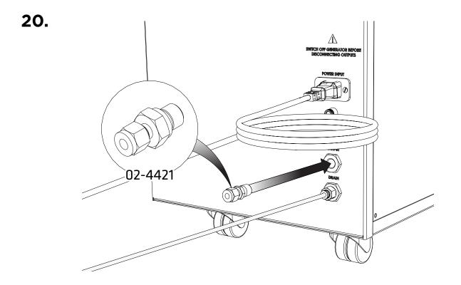
Depending on the size of the inlet on the instrument, select either the ¼" Compression Fitting 02-4421 or the remaining ¼"- 6mm Push Fit Fitting 02-4600 and attach this to the Nitrogen port.
