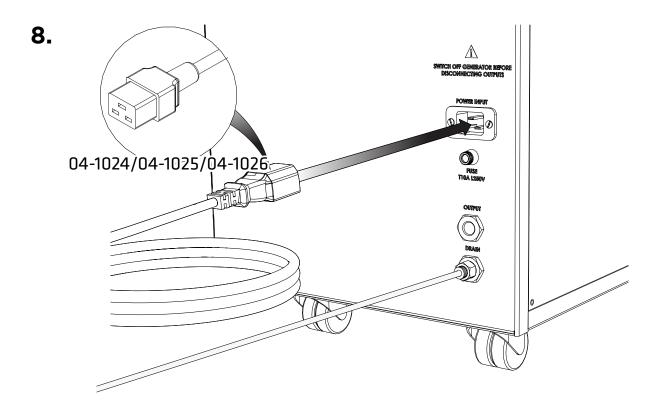
Select the appropriate mains cable from the fittings kit and plug the **IEC 60320/C19** cable into the mains input at the rear of the generator.
