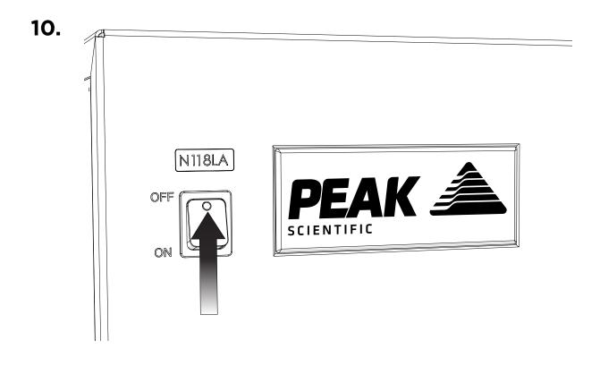
Switch the generator **ON** using the switch on the front panel.
