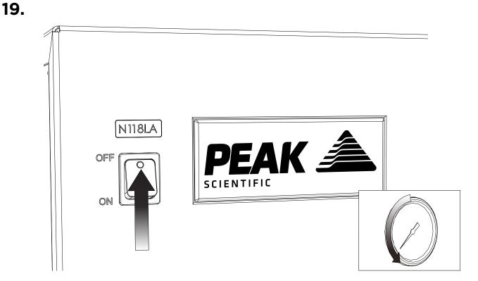
The purge is now complete, switch the generator **OFF** using the switch on the front panel. Once the **pressure gauge** reads **O**, the installation can continue.
