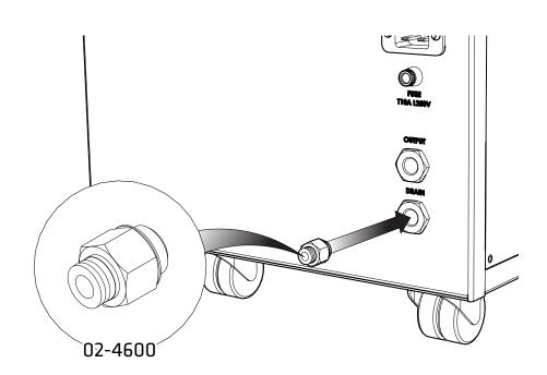
Select the ¼"- 6mm Push Fit Fitting 02-4600 and attach to the Drain port at the rear of the generator.
