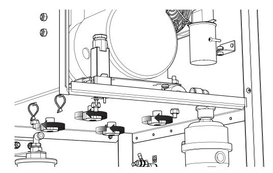
Remove the four thumb-screws and shake-proof washers from the underside of the compressor compartment. Then lift each transit bracket up until the locating pin an threaded stud are clear of the mounting plate and the compartment floor.
