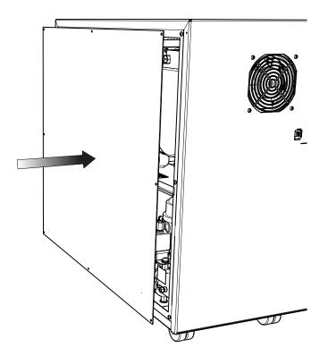
**Reattach** the side panel ensuring the **earth lead is re-connected** and the panel is fastened securely.
