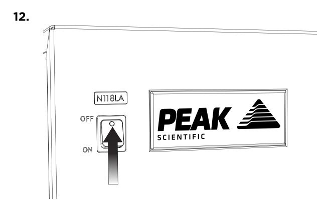
Switch the generator **OFF** using the switch on the front panel.
