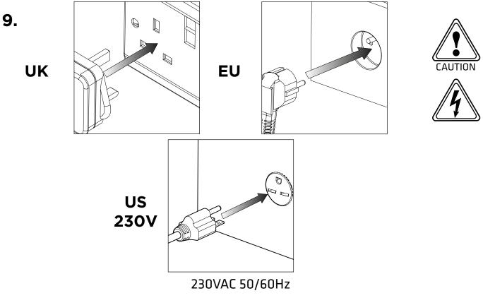
Plug the mains cable into the corresponding **230VAC 50/60Hz** single phase power supply.
