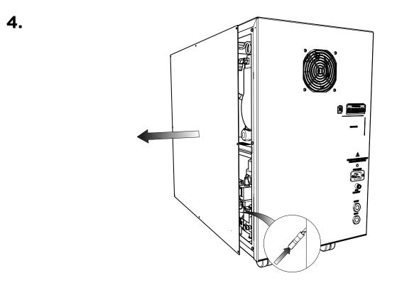
The side panel can now be **removed**, an **earth lead** is connected to the inside of the panel. This can be **disconnected** by pulling it off the spade connector on the panel.
