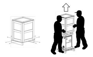
The generator can now be lifted out of the crate base and onto the floor. This should be done again with someone positioned at either side. There is a gap in the foam base for hand access; one hand should be positioned here underneath the generator and the other at the back supporting the weight. The generator should then be tilted back slightly and then up and out of the foam base and onto the floor.
