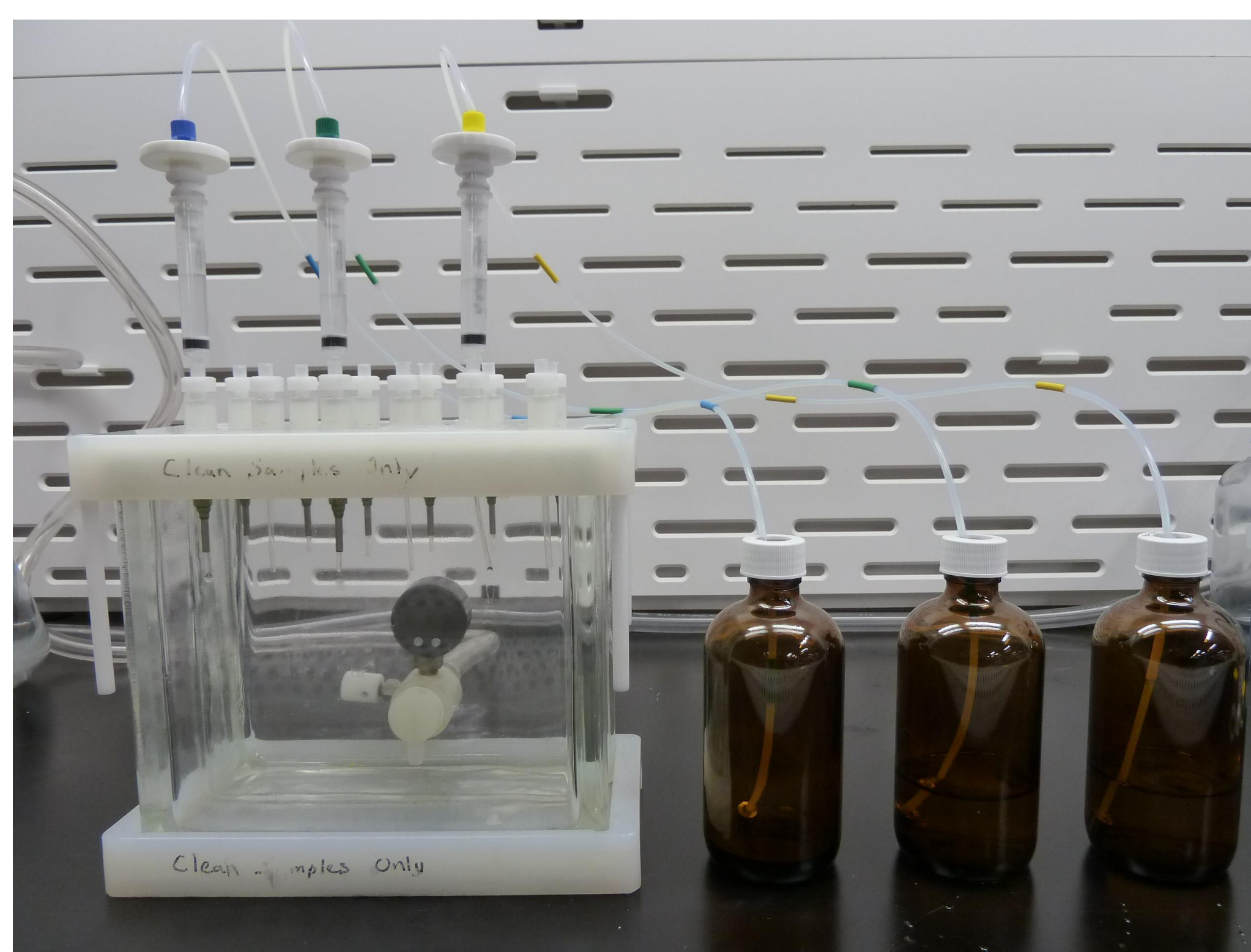
Figure 2. A 12-port vacuum manifold with sample delivery system was employed for the SPE extraction of pesticides
