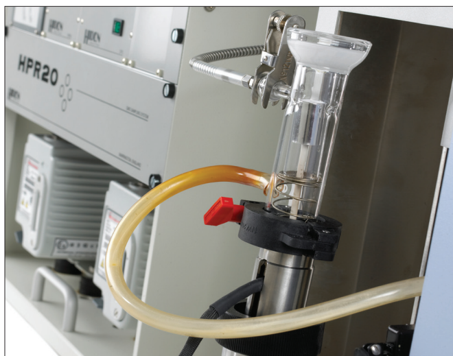
Figure 2. TGA low-mass platinum microfurnace.
