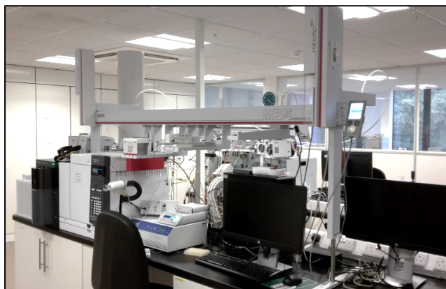
Figure 1: MPS Robotic Dual Head equipped with DHS and ODP and coupled to Agilent GC/Q-TOF.
