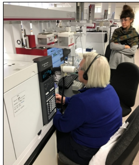
Figure 5: Mrs Joy Milne sniffing out PD relevant chromatographic peaks using the GERSTEL Olfactory Detector Port (ODP).
