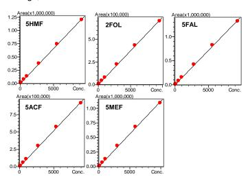
Fig 2. Calibration curves of furanic compounds standards (50 μg/L ~ 9000 μg/L), each pre-spiked in transformer oil
