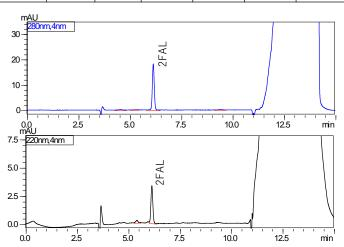
Fig 3. HPLC chromatogram of transformer oil sample TO6
