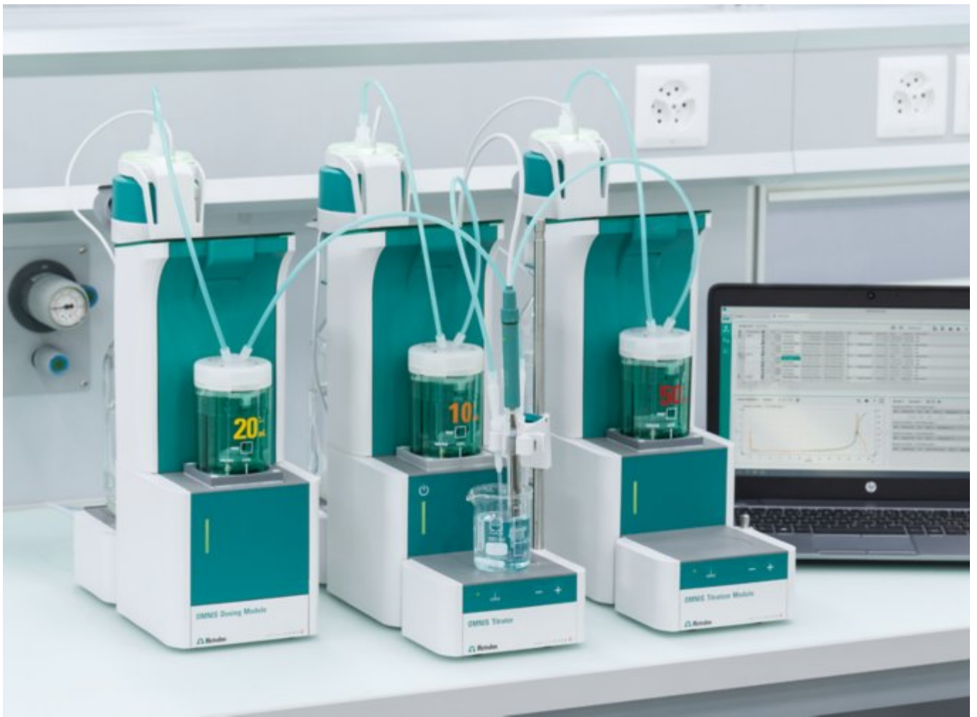
Figure 2. OMNIS Titrator equipped with a dSolvotrode electrode for the determination of caffeine content in nonaqueous samples.
