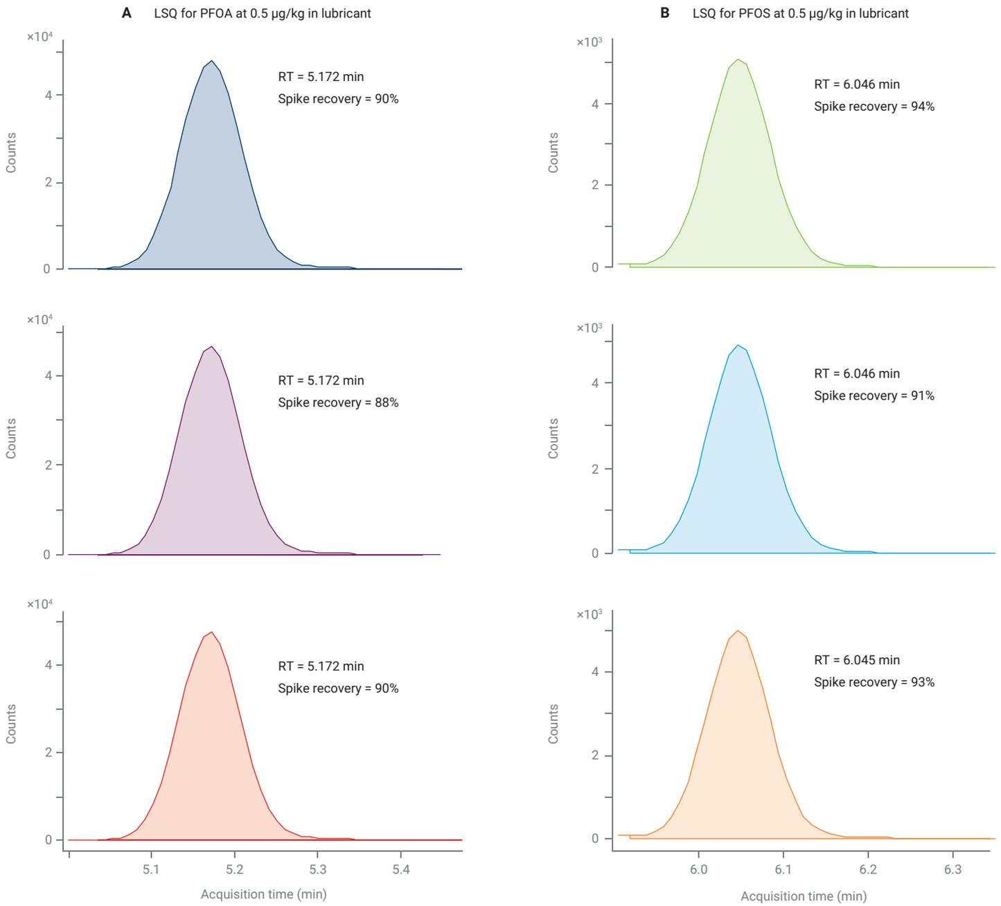
**Figure 3.** The chromatogram overlay of triplicate preparations of LSQ for PFOA (A) and PFOS (B) at 0.5 µg/kg.
