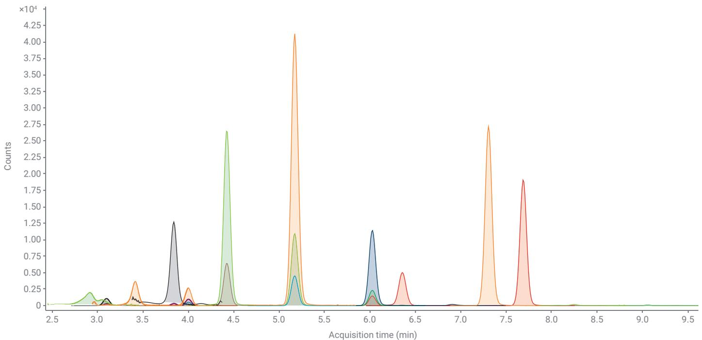
**Figure 4.** The MRM chromatogram of the unspiked lubricant sample extract (matrix blank).
