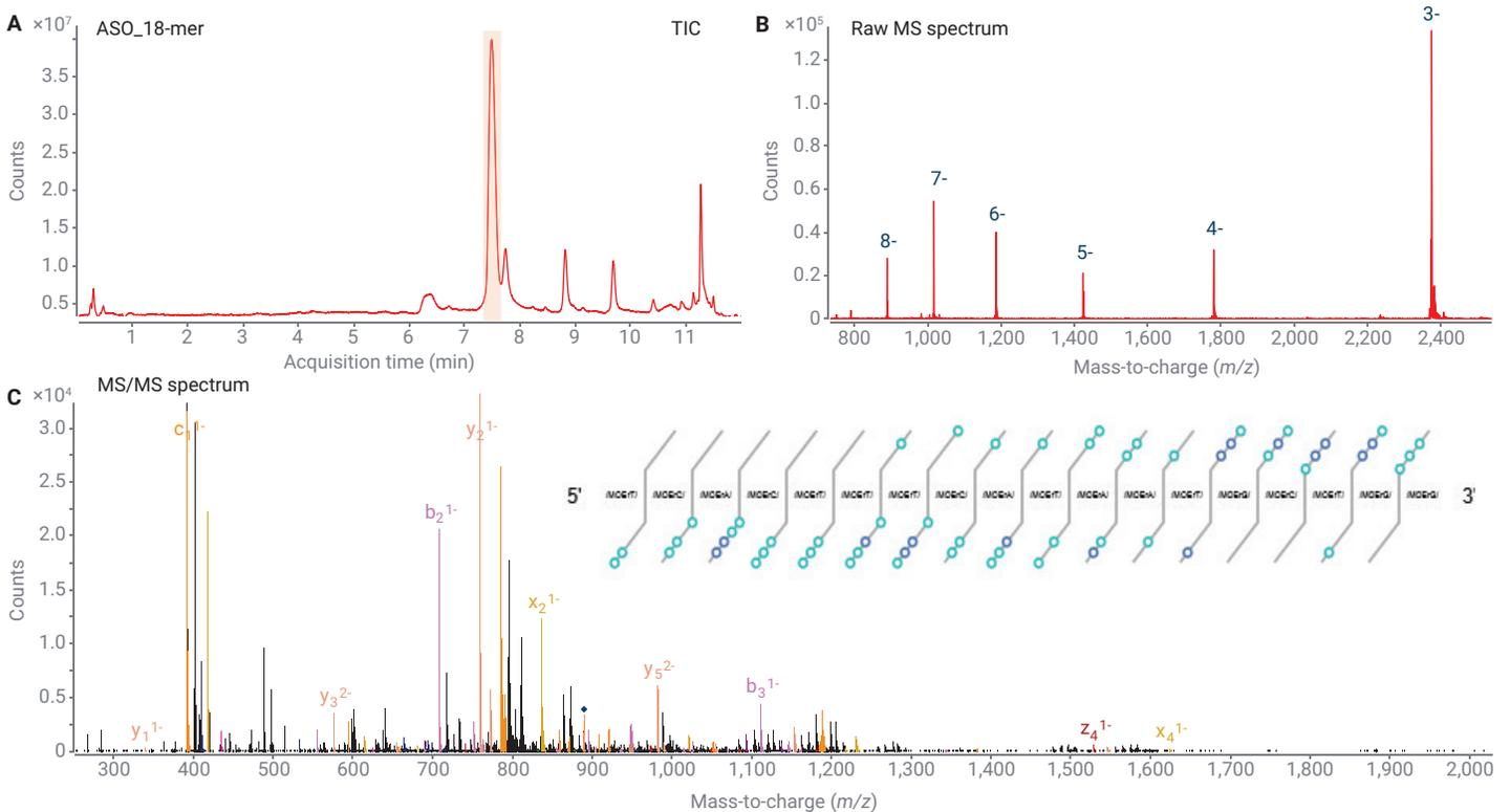
**Figure 10.** LC/MS/MS analysis on oligonucleotide with specific modifications (ASO\_18-mer). (A) Total ion chromatography (TIC) of ASO\_18-mer. (B) Raw MS spectrum of ASO\_18-mer. (C) MS/MS spectrum of ASO\_18-mer with Fragment Confirmation Ladder displayed.
