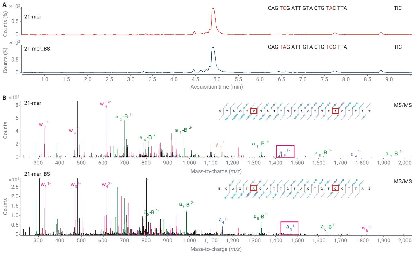
**Figure 7.** LC/MS/MS analysis on synthetic oligonucleotides (21-mer and 21-mer BS). Top two panels: Total ion chromatography (TIC) of the 21-mer and 21-mer BS (base swap) oligonucleotides. Bottom two panels: MS/MS spectrum of the 21-mer and 21-mer BS oligonucleotides.
