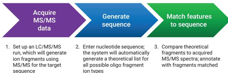
**Figure 2.** Oligonucleotide Sequence Confirmation data analysis workflow in Agilent MassHunter BioConfirm software, version 12.0.
