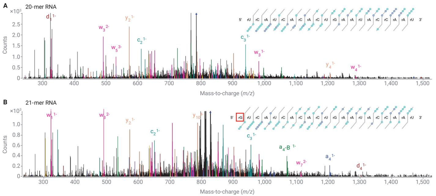
**Figure 6.** LC/MS/MS analysis on the Agilent oligonucleotide (RNA) resolution standard (20-mer and 21-mer). MS/MS spectrum of 20-mer and 21-mer RNA with Fragment Confirmation Ladder displayed.
