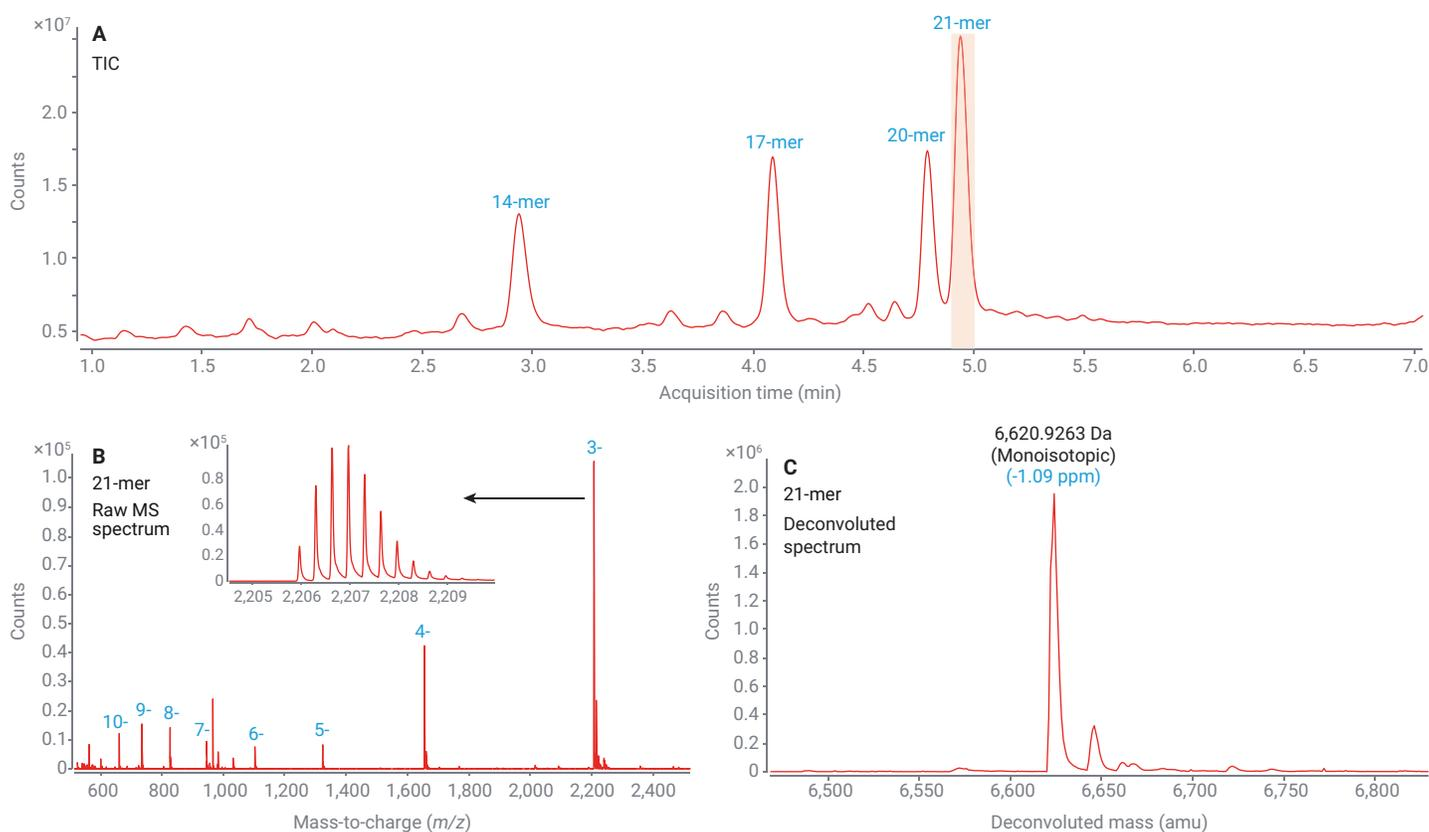
**Figure 3.** LC/MS analysis of Agilent oligonucleotide (RNA) resolution standards. (A) Total ion chromatography (TIC) of the resolution standards. (B) Raw MS spectrum of the selected 21-mer RNA. (C) Deconvoluted MS spectra of the 21-mer RNA standard.
