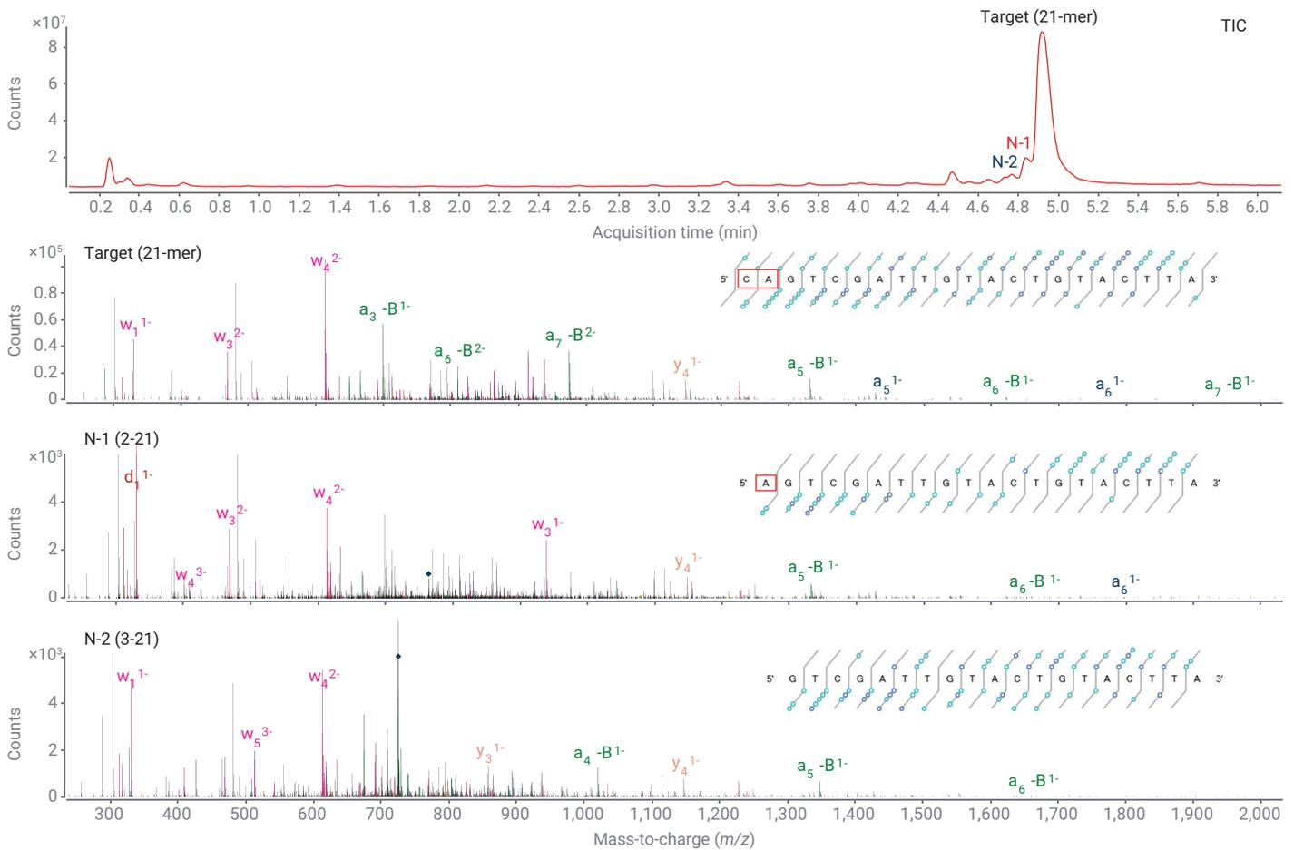
**Figure 11.** Oligonucleotide sequence confirmation of full-length target (21-mer) and the N-1 (2-21) and the N-2 (3-21) impurities.
