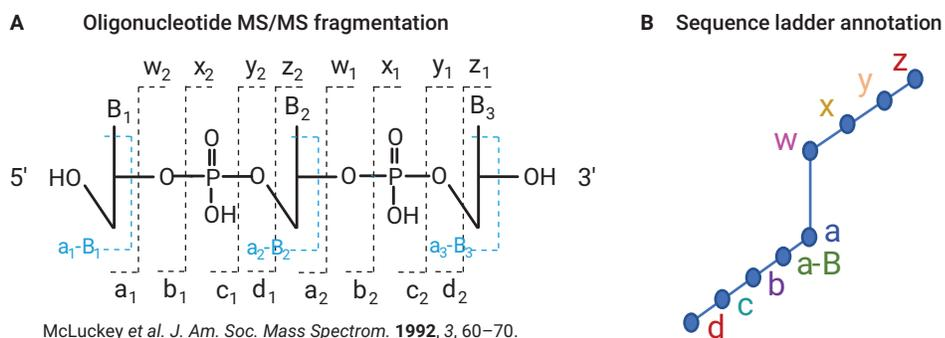
**Figure 4.** Nomenclature of oligonucleotide fragmentation (A) and annotation for oligonucleotide Fragment Confirmation Ladder (B). The colors of letters represent the different types of fragment ions identified and labeled in the MS/MS spectra.
