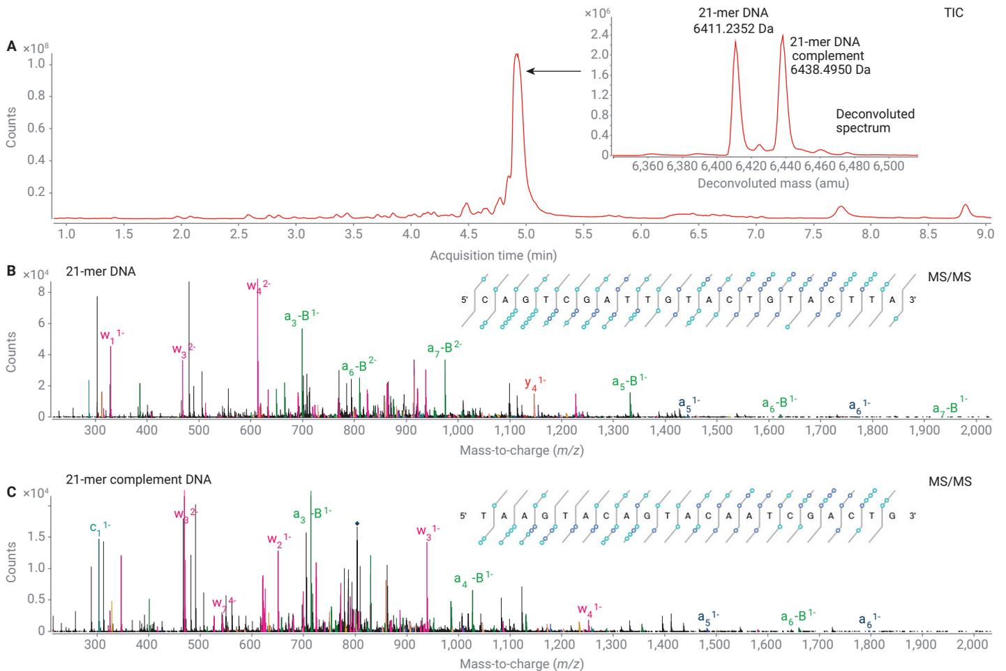
**Figure 9.** LC/MS/MS analysis of double-stranded DNA (21-mer and 21-mer complement). (A) Total ion chromatography (TIC) of double-stranded DNA (21-mer and 21-mer complement). (B) and (C) MS/MS spectrum of double-stranded DNA (21-mer and 21-mer complement).
