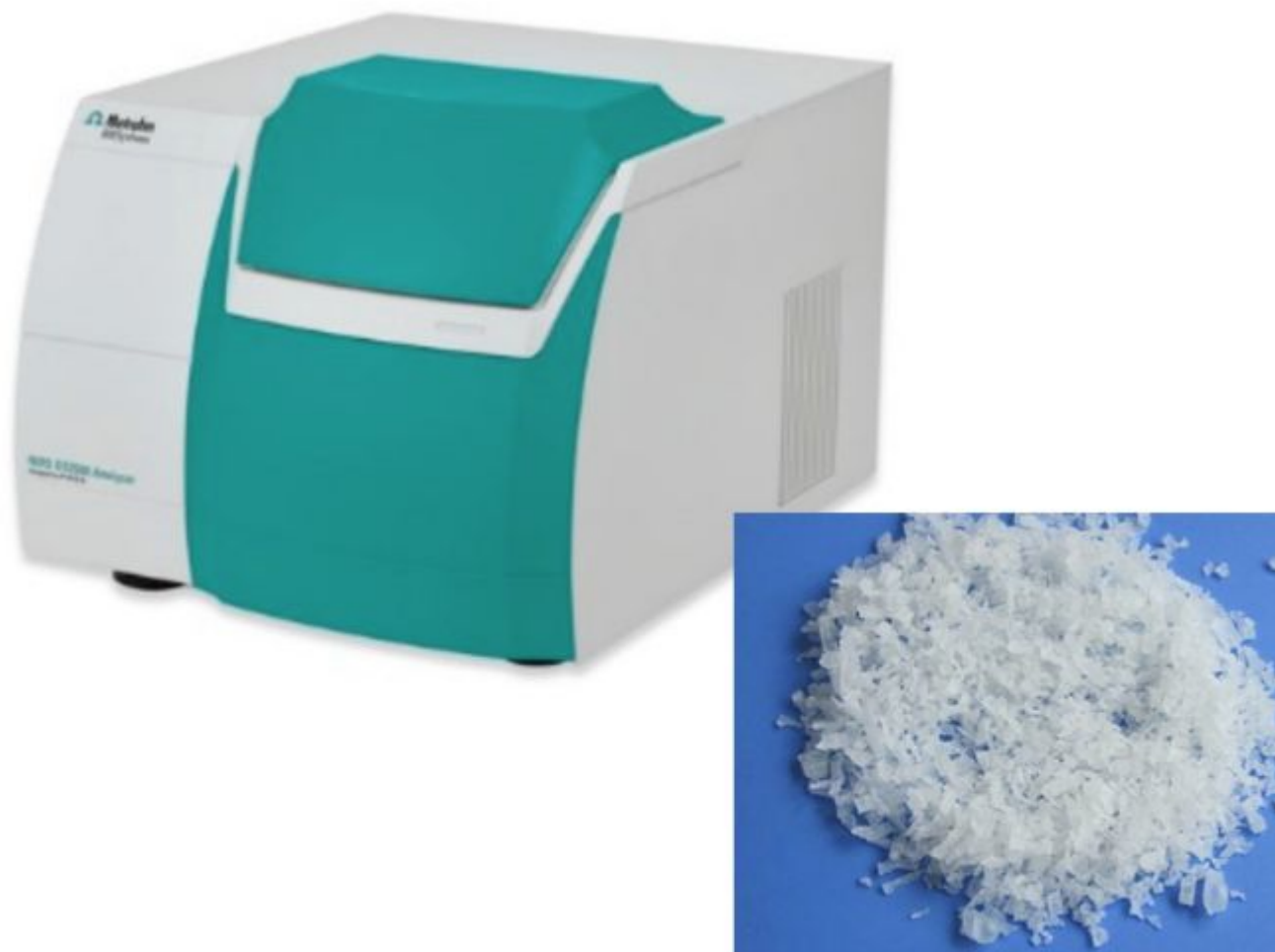
Figure 1. The DS2500 Solid Analyzer was used to collect the spectra of PVA polymer.
