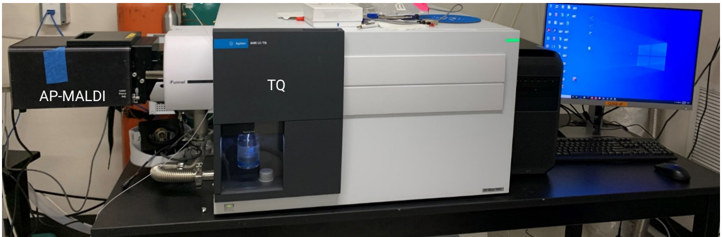
Figure 1. MassTech AP-MALDI ion source and Agilent 6495 triple quadrupole systems.
