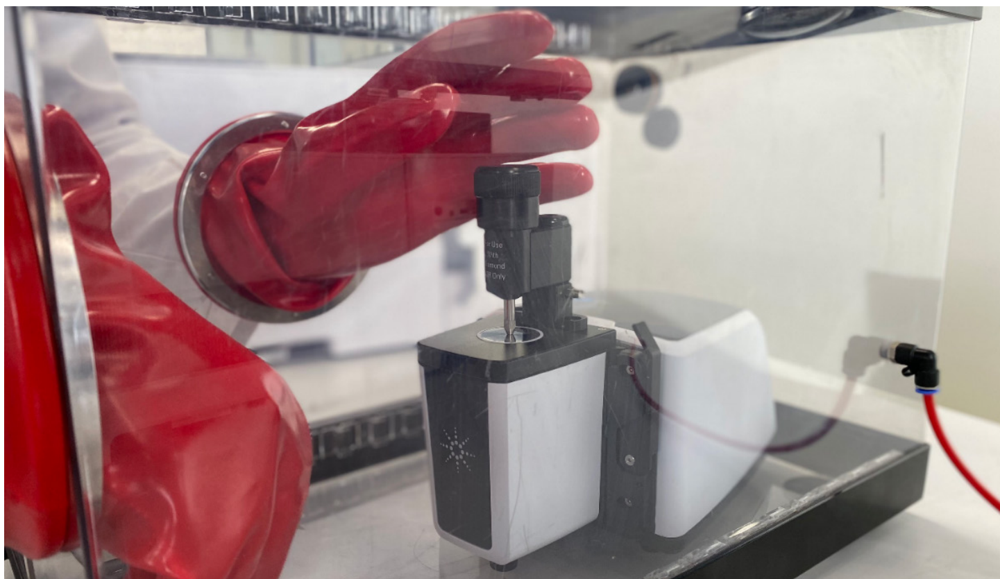
Figure 1. The Agilent Cary 630 FTIR spectrometer with its ultracompact, lightweight design (20 × 20 cm and 3.6 kg) can easily be used in a glove box to produce high-quality results.
