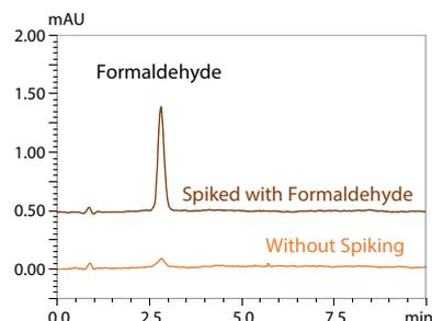
**Fig. 8 Chromatogram of Hair Conditioner (Dissolved in Water/THF=50:50)**
