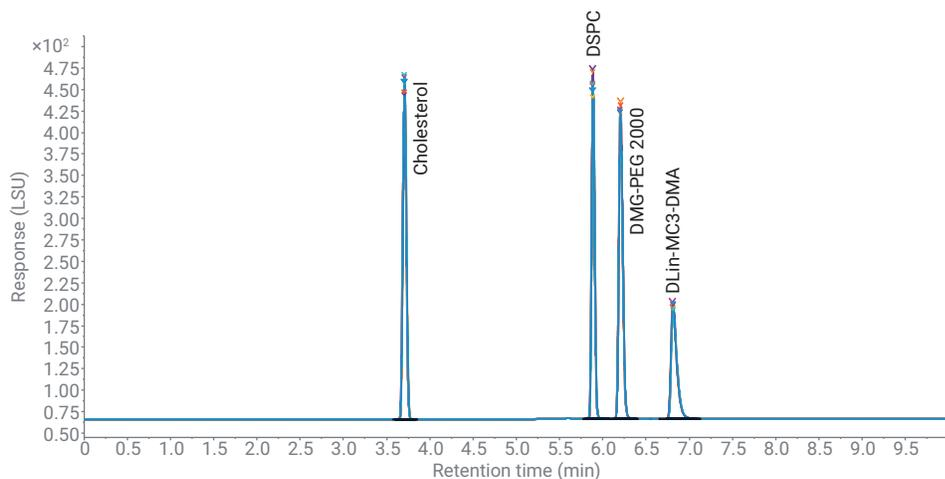
**Figure 7.** Quaternary gradient using MeOH as well as ACN – Overlay of seven subsequent runs.
