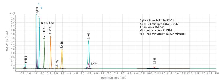
**Figure 3.** Agilent 1260 Infinity II Binary HPLC System, premix (buffer: 5.4 g/L of monobasic potassium phosphate. Adjust with phosphoric acid to a pH of 3.0. Mobile phase: acetonitrile and buffer (35:65) 1.5 mL/min 220 nm, 4 µL injection.
