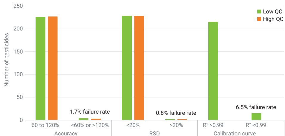
Figure 8. Method verification results summary for quantitative determination of 230 pesticides in mixed bell pepper by LC/MS/MS and GC/MS/MS. Samples were prepared using the Agilent Bond Elut QuEChERS AOAC extraction kit followed by Agilent Captiva EMR–GPF passthrough cleanup.
