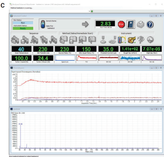
Figure 7. The novel leak testing tool that enables monitoring of the user-specified ions to identify the source and the amount of leak.
