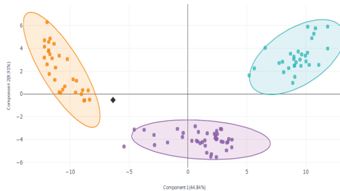
Figure 7. Classifier 1.0 results for (A) QC sample and (B) adulterated black pepper sample at 50:50 ratio. (C) Adulterated black pepper sample at 70:30 ratio. The Phu Quoc class is orange, the Binh Phuoc class is purple, and the DakLak class is teal. The black diamond represents the selected sample.
