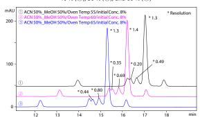
Fig. 6 Chromatograms with Different Column Oven Temperature 55 °C (①), 60 °C (②), and 65 °C (③)
