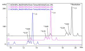
Fig. 5 Chromatograms with Different Acetonitrile Ratio 40 % (①), 50 % (②), and 60 % (③)
