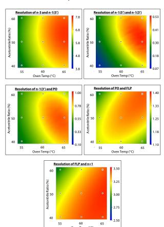
Fig. 11 Design Space for Resolution of FLP and Related Impurities (Initial concentration is 8 %.)
