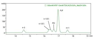
Fig. 4 Chromatogram of Highest Evaluation Value (Enlarged Chromatogram of Fig. 2 ⑤)
