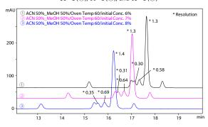
Fig. 7 Chromatograms with Different Initial Concentration 6 % (  $\^{\ }$  ), 7 % (  $\^{\ }$  ), and 8 % (  $\^{\ }$  )
