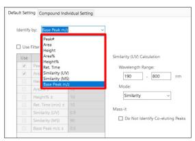
Fig. 10 Parameter Setting for Peak Tracking with LabSolutions MD
