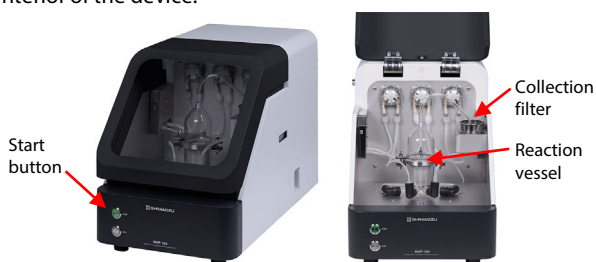
Fig. 1 (Left) External Appearance and (Right) Interior of MAP-100
