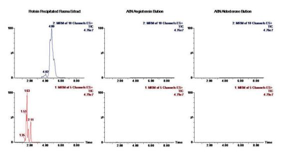
Figure 3. Phospholipid profile comparison between protein precipitated serum and optimized SPE extracts using ethyl acetate and 2% NH<sub>4</sub>OH in 50/50 (v/v) MeOH/H<sub>2</sub>O as elution solvents.
