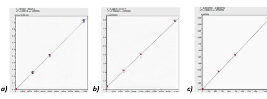
Figure 5. Calibration curves for Angiotensin I (a), Angiotensin II (b), Aldosterone (c) using plasma containing K2 EDTA anti-coagulant.
