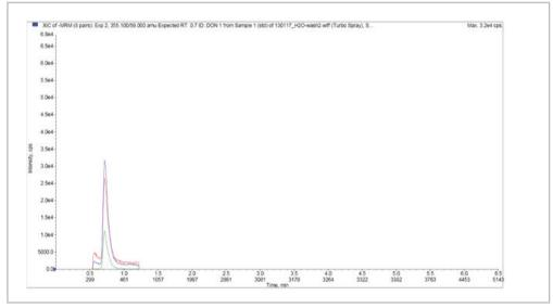
Figure 2. Extracted ion chromatogram for deoxynivalenol in negative ion mode using ISOLUTE® protocol at 100  $\mu g \ kg^1$  from wheat
