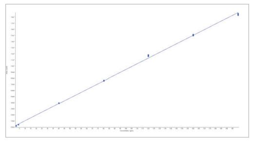
Figure 3. Calibration curve for deoxynivalenol from ground wheat using the ISOLUTE $^{\otimes}$  Myco protocol from 2–200 ng mL $^{1}$
