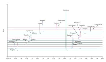
Figure 1. Separation of 23 drugs of abuse under 4 minutes on the Accucore Biphenyl column
