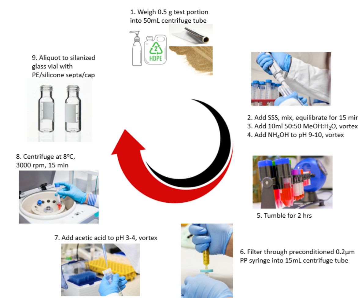
Figure 2. Sample preparation procedure for consumer products
