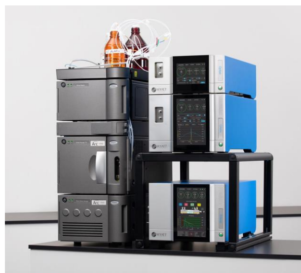
Figure 1. An FFF-MALS-DLS system comprising autosampler and pump (bottom left), Eclipse FFF instrument and separation channel (bottom right, foreground), and three detectors: UV (top left), MALS/DLS and refractive index (top right).
