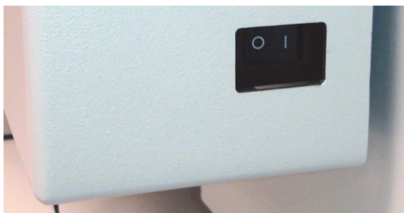
Figure 6. Power switch on the lower right side of the ion source
