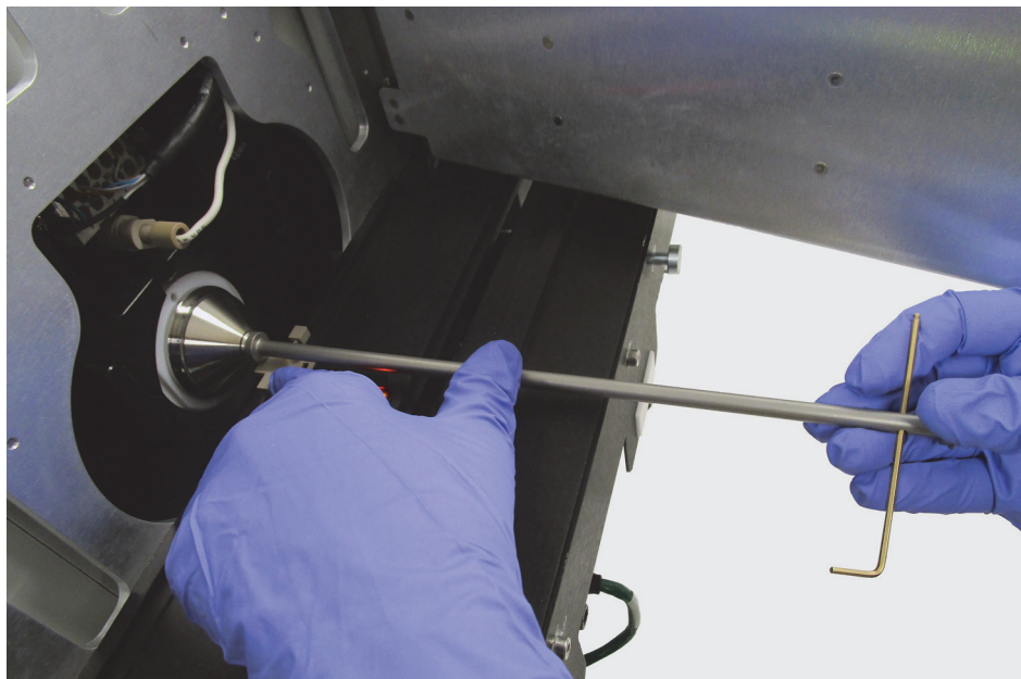
Figure 50. Releasing the ion transfer tube from the spray cone
