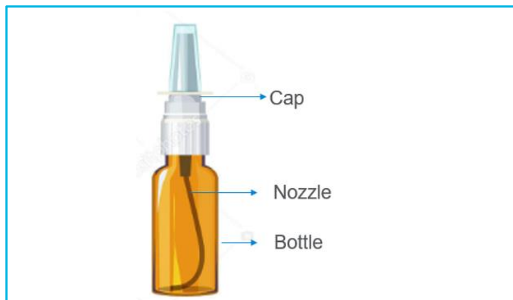
Figure 1. Drug container closure system
