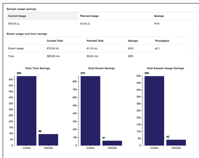
Figure 14. The absolute values for analysis time, eluent usage, and sample usage of the current and planned method are calculated by the HPLC Method Transfer Calculator. The savings of eluent, sample, and time due to the method transfer are highlighted.
