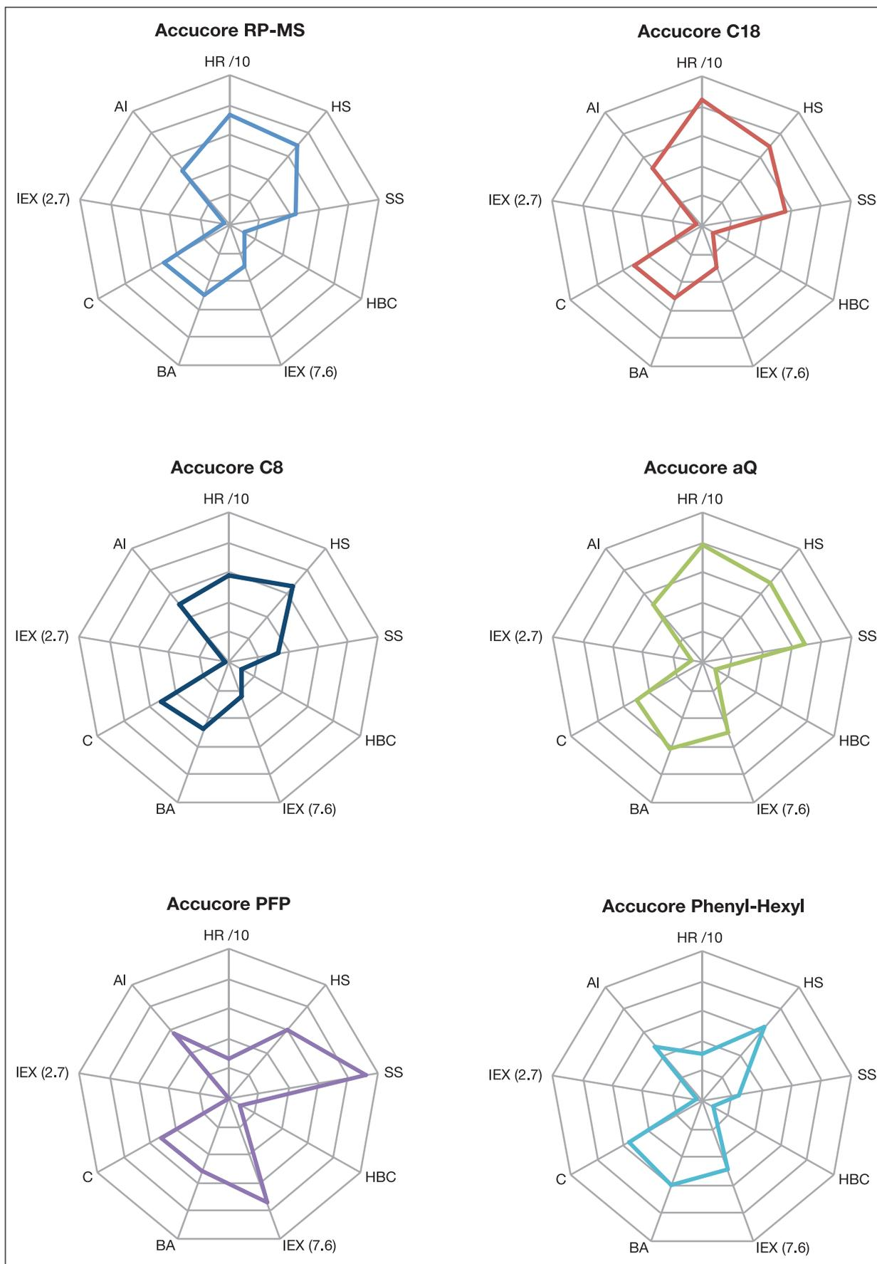
Figure 2: Summary of differences in selectivity offered by Accucore columns. HR= hydrophobic retention; HS= hydrophobic selectivity; SS= steric selectivity; HBC= hydrogen bonding capacity; IEX (7.6)= ion exchange capacity at pH 7.6; BA= activity towards bases; C= activity towards chelators; IEX (2.7)= ion exchange capacity at pH 2.7; AI= activity towards acids.
