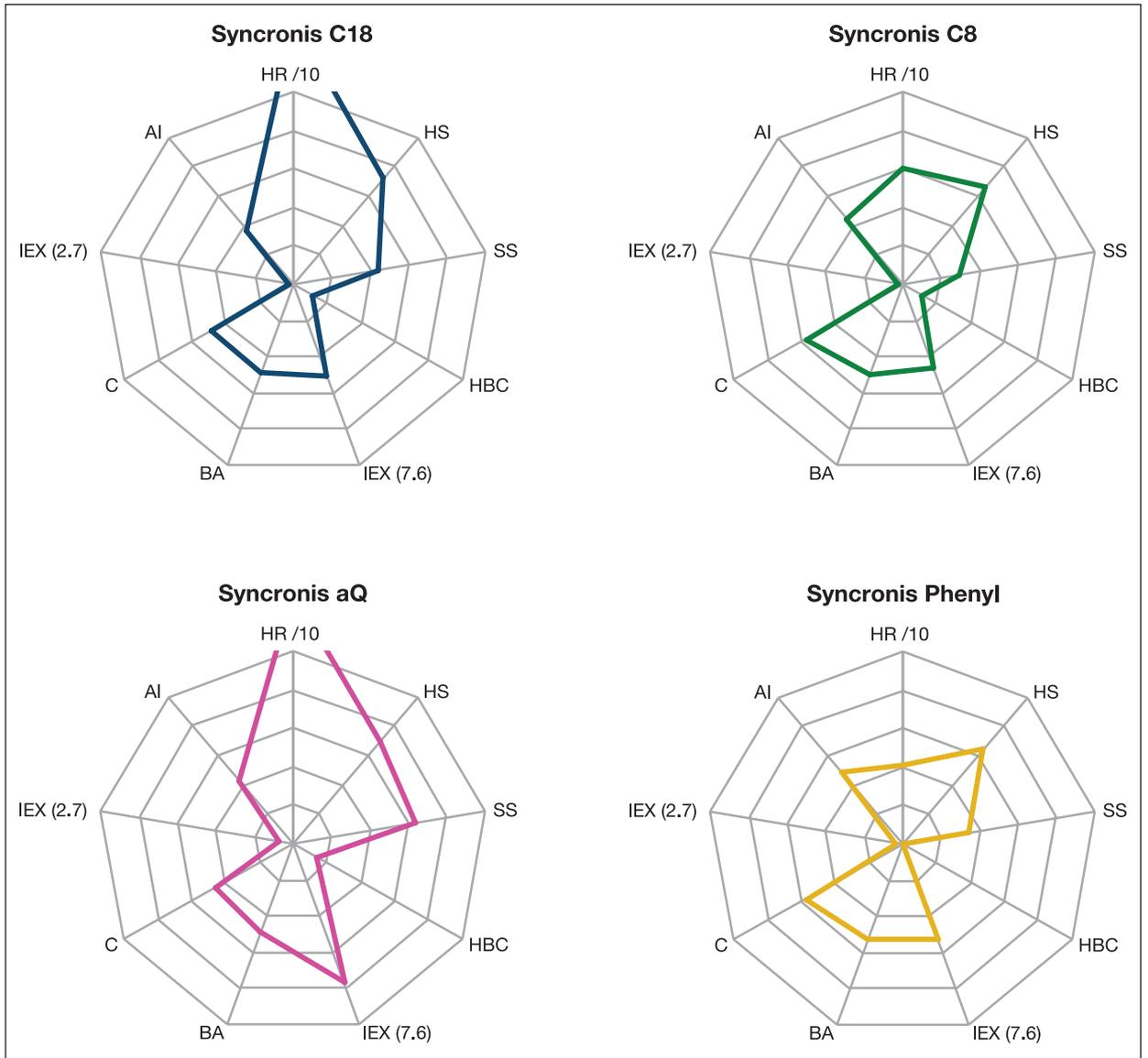
Figure 4: Summary of differences in selectivity offered by Synchronis columns. HR= hydrophobic retention; HS= hydrophobic selectivity; SS= steric selectivity; HBC= hydrogen bonding capacity; IEX (7.6)= ion exchange capacity at pH 7.6; BA= activity towards bases; C= activity towards chelators; IEX (2.7)= ion exchange capacity at pH 2.7; AI= activity towards acids.
