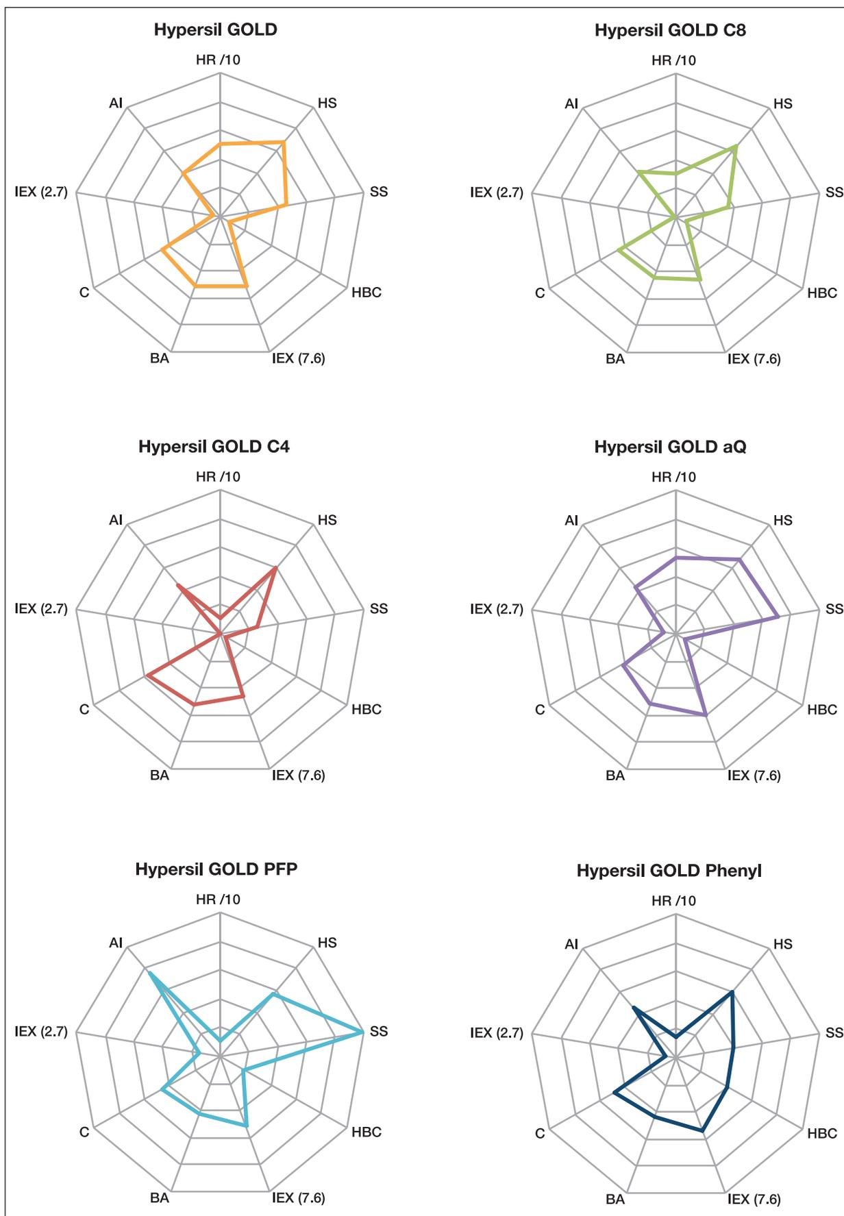
Figure 3: Summary of differences in selectivity offered by Hypersil GOLD columns. HR= hydrophobic retention; HS= hydrophobic selectivity; SS= steric selectivity; HBC= hydrogen bonding capacity; IEX (7.6)= ion exchange capacity at pH 7.6; BA= activity towards bases; C= activity towards chelators; IEX (2.7)= ion exchange capacity at pH 2.7; AI= activity towards acids.
