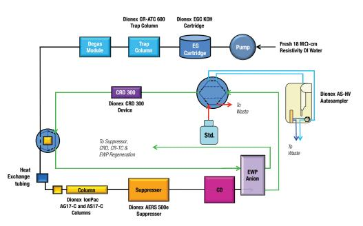
Figure 1. Flow diagram of Dionex Integrion HPIC system for trace anion determinations.
