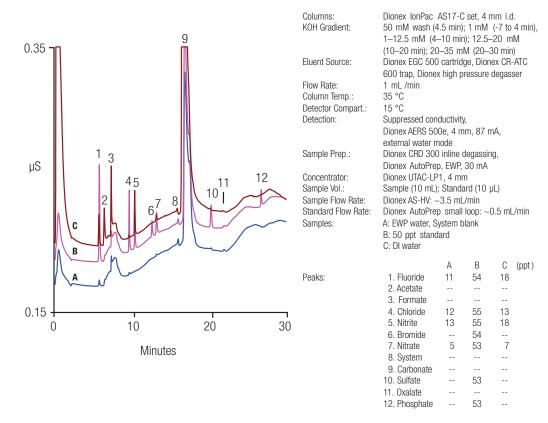
Figure 14. Comparison of the system blank, DI water, and a 50 ppt standard.
