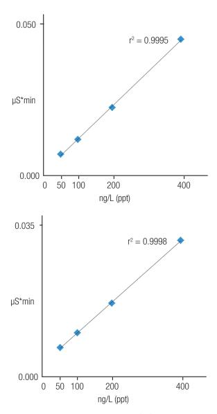
Figure 12. Calibration curves for chloride (top) and sulfate (bottom).
