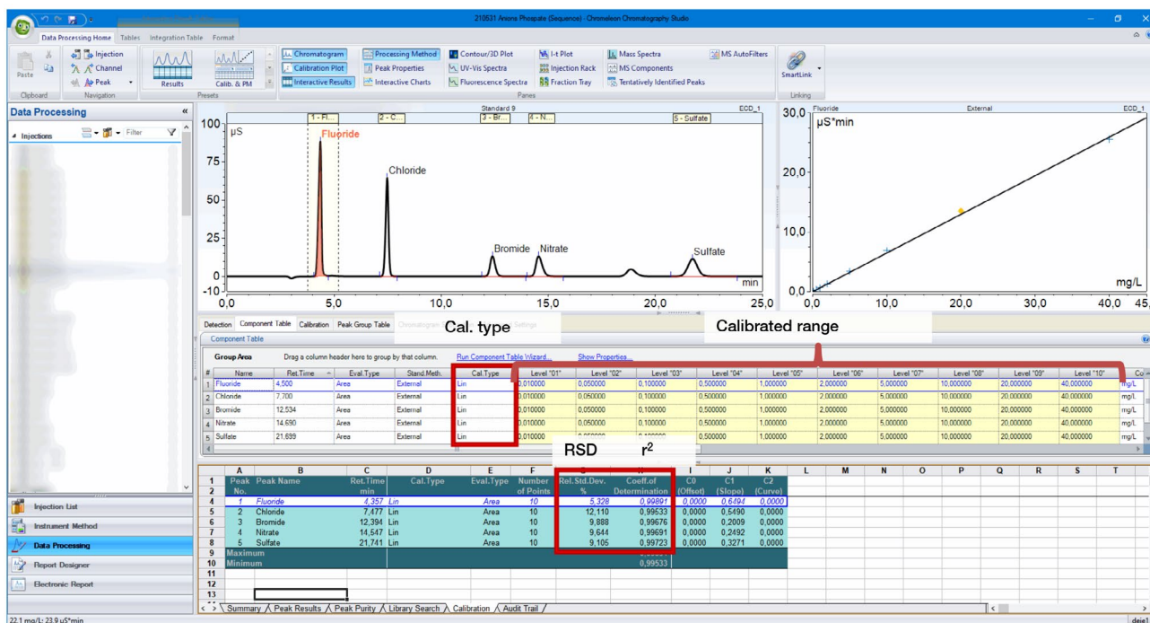
Figure 1. Chromeleon CDS Studio View illustrates anion separation on a Dionex IonPac AS23 column. Eluent used: 4.5 mM \text{Na}_2\text{CO}_3/0.8 mM \text{NaHCO}_3 with a flow rate of 1 mL/min and an injection volume of 50 \mu\text{L} . Detection was performed with suppressed conductivity using a Thermo Scientific™ Dionex™ ADRS600 Suppressor, and data were acquired at a rate of 5 Hz. The standard concentration was 20 mg/L for each ion, with the processing method and calibration report shown in the default layout.
