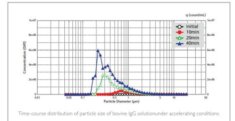
Application News: Evaluation of Protein Aggregation Under Various Stress Conditions Using the Aggregates Sizer
