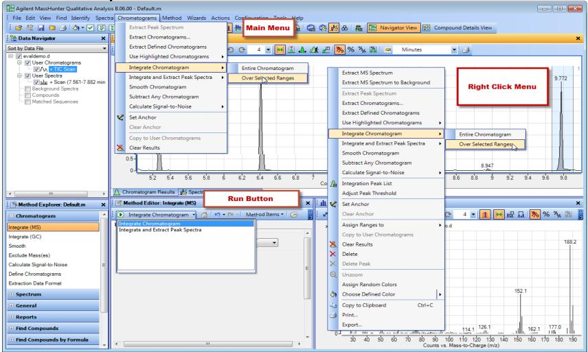
Set parameters for action in Method Editor. Then, perform action. Note : The action will be performed on ALL selected (highlighted) items!
