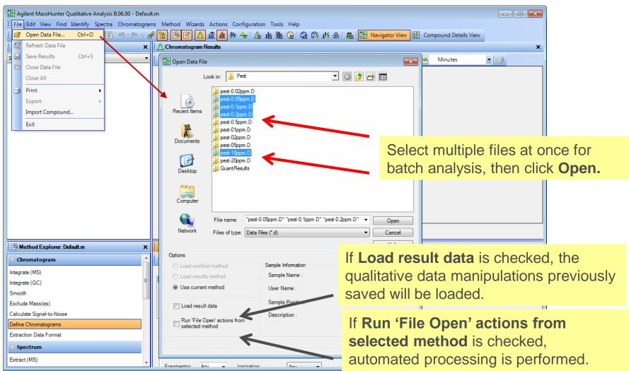
If neither **Load result data** or **Run 'File Open' actions from selected method** is checked, then a TIC is automatically extracted from the data files.
