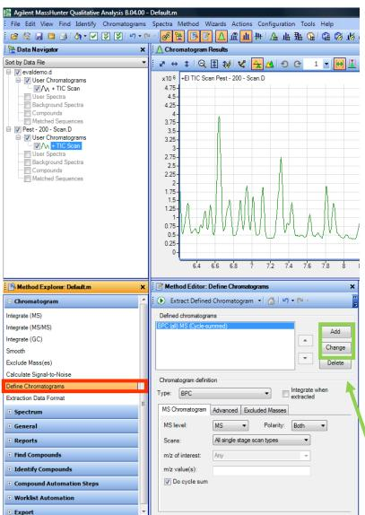
• Select MS Level based on acquisition scan type.
