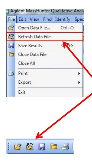
Feature is useful when it is desired to view data as the data file is being acquired.
