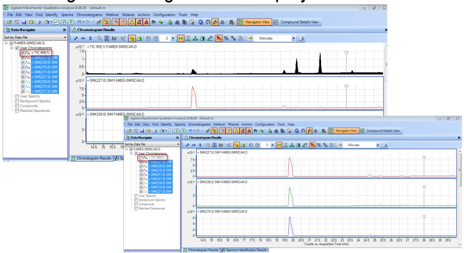
Items in the Data Navigator, like Chromatograms, will be displayed if checked and not displayed if unchecked.
