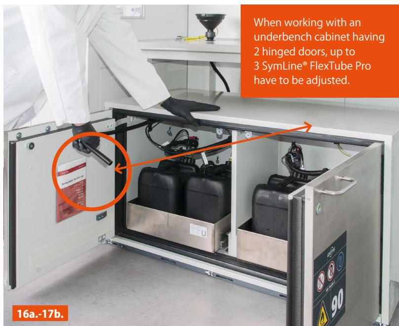
When working with an underbench cabinet having 2 hinged doors, up to 3 SymLine<sup>®</sup> FlexTube Pro have to be adjusted.
