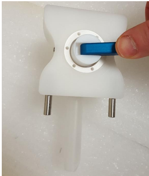
Figure 8-1. Using the supplied WIV to Rotate the Valve
