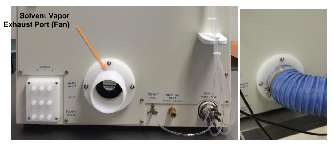
Figure 5-6. Exhaust port at the bottom rear of the Biotage® Horizon 5000. Photo on the right shows the Exhaust Hose installed
