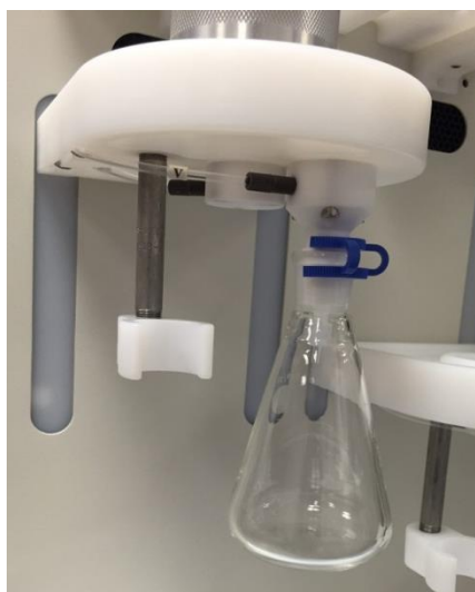
Figure 6-41. Loading the Collection Vessel
