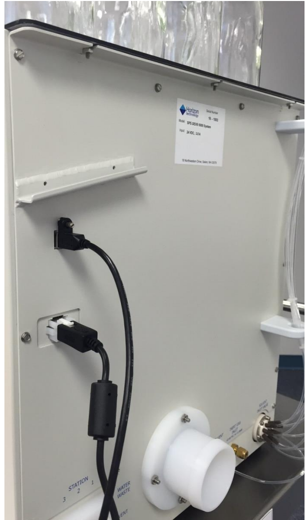
Figure 5-8. PC Communication Cable Connected to the PC Communication Port
