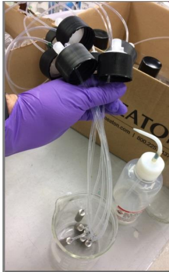
Figure 8-3. Solvent Line Sinkers being Cleaned
