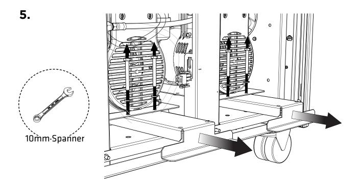
The transit brackets are located below the compressors and have stickers on them stating 'Remove before use'. To **remove the transit brackets**, use a **10mm spanner** to **remove the two screws on each bracket** as indicated, then **slide the brackets out** from underneath the compressors. **There are three brackets in total. Please retain** the brackets and screws for future transportation.
