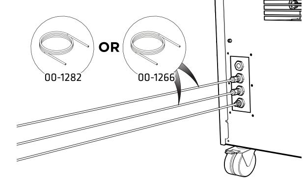
Attach the appropriate sized **tubing** to the fitting attached to the **Nitrogen and Air ports** and connect the other end to the **gas inlet of your instrument**.
