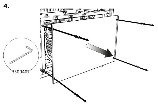
With the right-hand side plate removed, use the **4mm Hex Key 3300407** to **remove the hex bolts** holding the compressor door in place, taking care to **retain the spring washers**.
