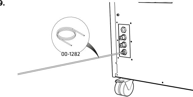
Connect the 6mm Polyethylene Tubing 00-1282 to the 6mm Push Fit Fitting 02-4600. Fit the other end of the tubing to a suitable drain connection or container. The container MUST NOT have an airtight seal as water and air will be expelled periodically under a slight pressure.
