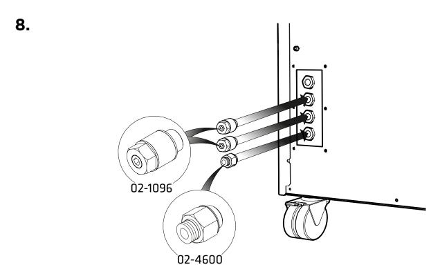
Select the 6mm Push Fit Fitting 02-4600 and attach to the Drain port at the rear of the generator. Attach the Flow Control Silencer 02-1096 to the Nitrogen and Air ports.
