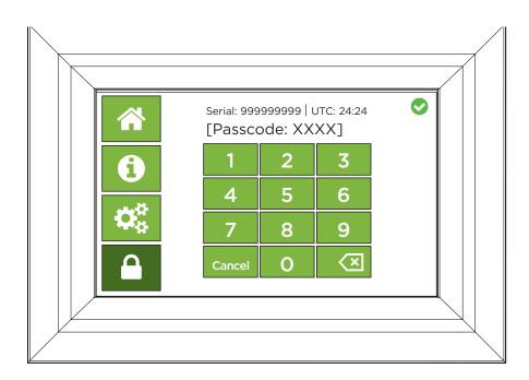
**Enter your PIN**. If entered incorrectly the screen will briefly display a wrong pass code warning before allowing a new PIN entry attempt.
