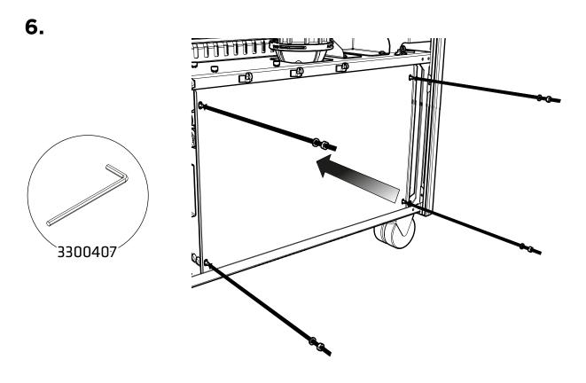
Replace the compressor doors, again using the 4mm Hex Key 3300407.
