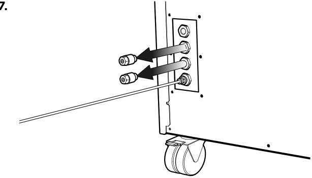
Once the pressure has dissipated the silencer fittings can be removed from the Nitrogen and Air ports.
