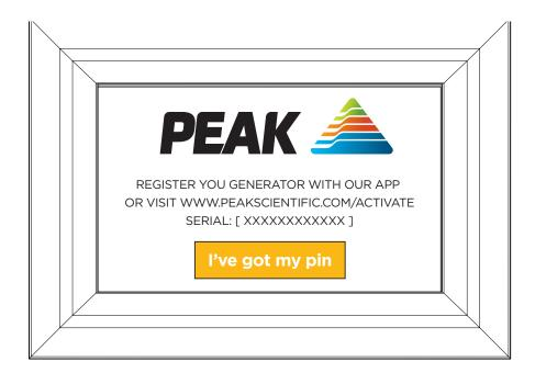
Before the generator will start-up for the first time the **user must enter a unique 4-digit PIN code.**
