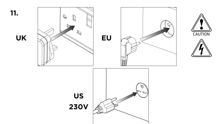
Plug the mains cable into the corresponding **230VAC 50/60Hz** single phase power supply.
