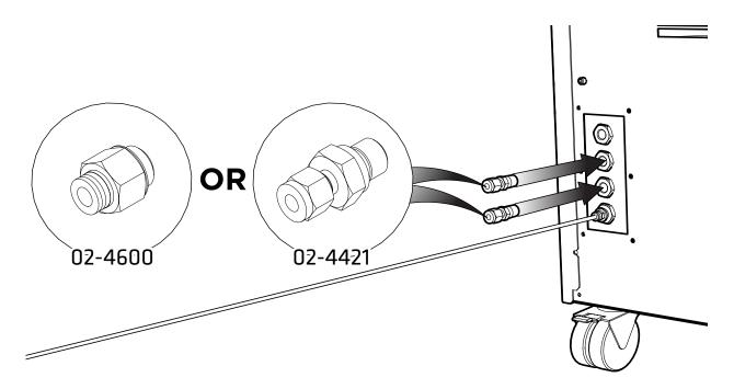
Depending on the size of the inlet on the instrument, select either the  $\frac{1}{4}$ " Compression Fitting 02-4421 or the remaining  $\frac{1}{4}$ "- 6mm Push Fit Fittings 02-4600 and connect these to the Nitrogen and Air ports.
