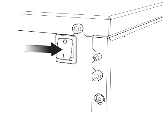
**After 30 minutes of running**, the generator can be turned **OFF**. Allow the stored gas in the internal tanks to dissipate.
