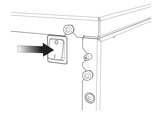
Switch the generator ON using the switch on the rear panel
