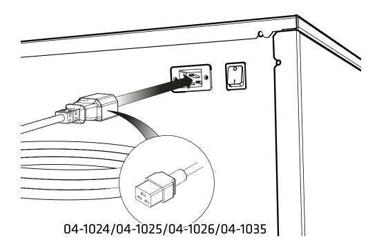
Select the appropriate power cable from the fittings kit and plug the IEC 60320/C19 cable into the power input at the rear of the generator.
