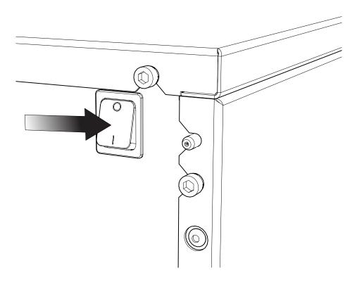
**Switch the generator ON** using the switch on the rear panel
