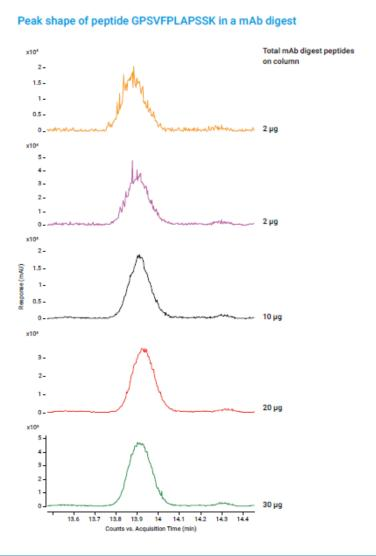
Peak shape comparison in 0.1% FA modified mobile phase at increasing sample loads
