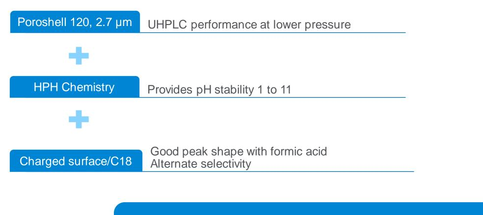
To make **AdvanceBio Peptide Plus** that provides sensitivity and resolution for accurate and robust identification and quantitation of biotherapeutic PTMs and synthetic peptide impurities when using formic acid as the mobile phase additive
