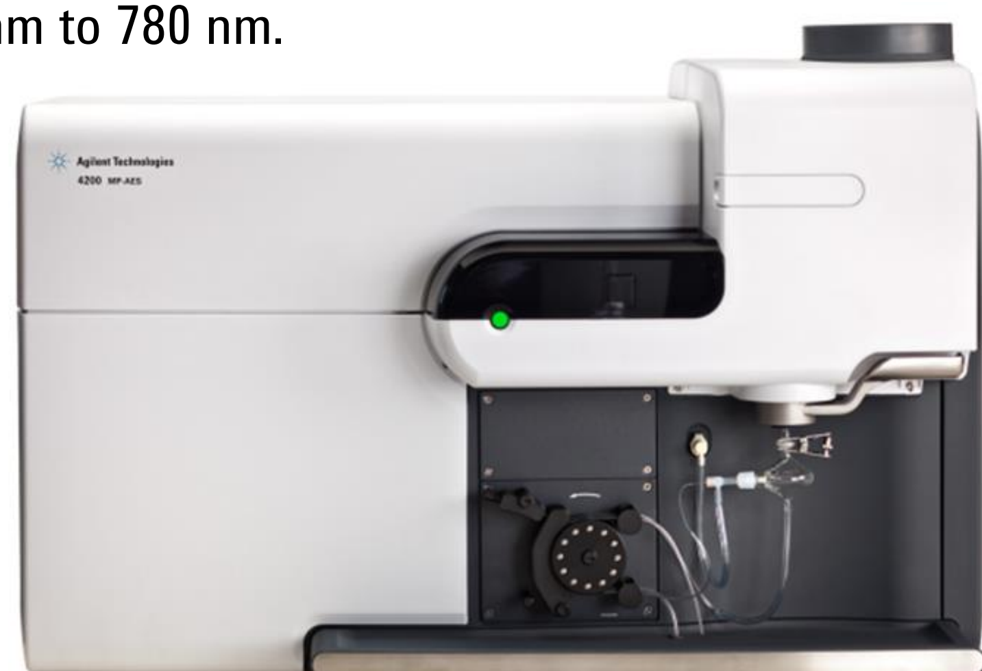
Figure 1. The Agilent 4200 MP-AES
