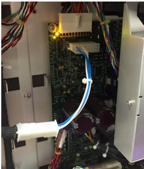
Figure 7. Heater assembly connection with ARC cable assembly on Agilent 7890 GC (electronics located behind plastic panel on detector side of GC).
