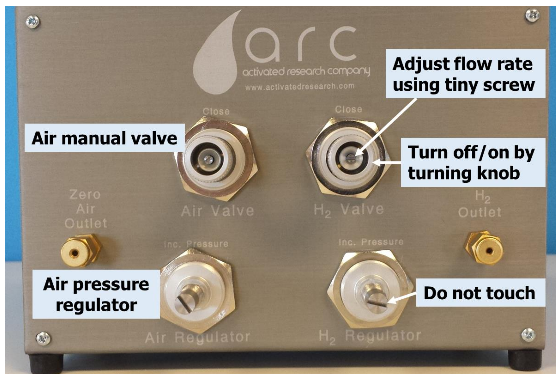
Figure A1. Schematic of manual flow control module.
