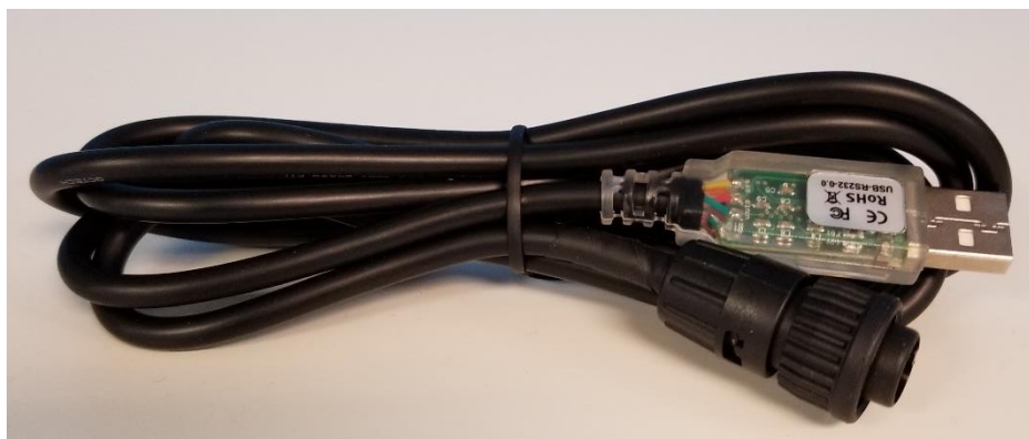
Figure A3. Schematic of EFC software communication cable.
