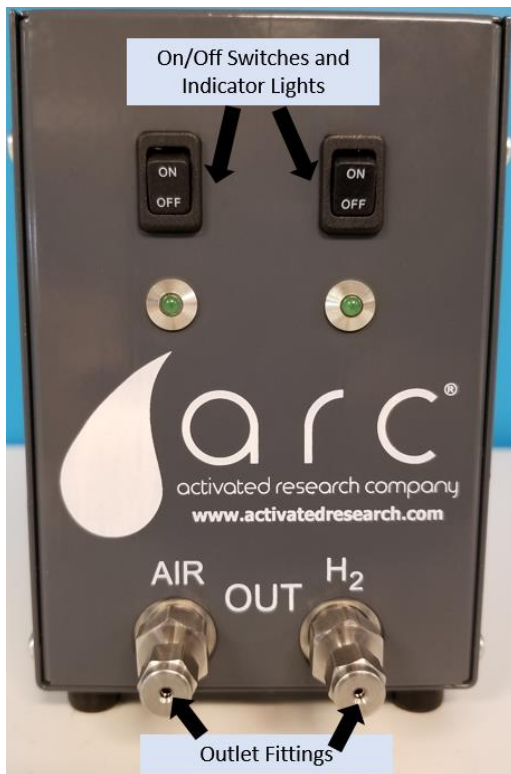
Figure A2. Schematic of front of electronic flow control module.
