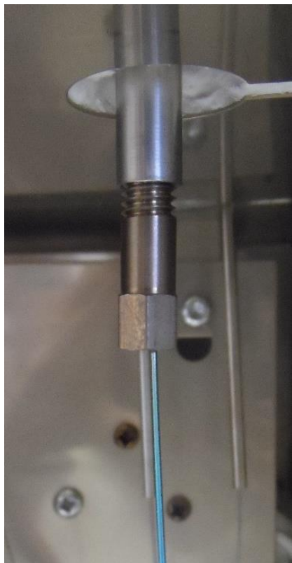
Figure 8. Outlet of the Polyarc® system inserted into the FID jet.
