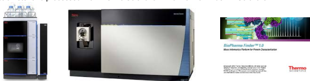
Figure 1. Data were collected using a Vanquish UHPLC coupled to an Orbitrap Fusion mass spectrometer and processed with Thermo Scientific™ BioPharma Finder™ Software.
