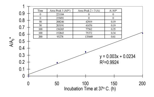
Figure 4 Fractional Amount of Deamidation Products Formed as a Function of Time when Ribonuclease A (3 mg/mL) was Incubated in 1% Ammonium Carbonate Buffer, pH 8.2, at 37 °C
