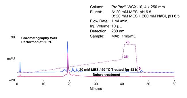
Figure 7 Effect of MES/50 °C Treatment on WCMAb Separation
