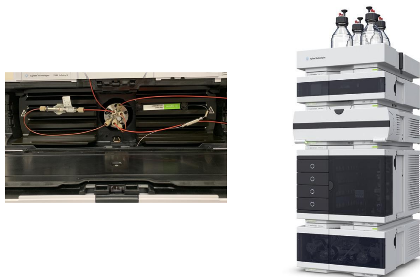
Figure 1. 10-port valve installed in column compartment, emulating a 6-port valve for diverting the salts and low MW species to waste.
