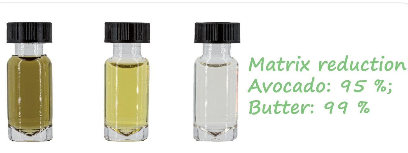
**Left**: Extract after addition of Mix I, **Middle**: Extract after dispersive SPE cleanup, Right: Extract after non-dispersive automated clean-up via FREESTYLE and Pesticide III QuEChERS column
