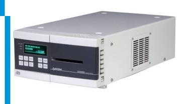
wavelength calibration after lamp start. High standard deuterium lamp in a special socket enables easy lamp exchange.
