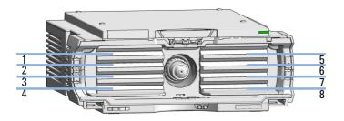
2 Connect the sampler outlet capillary (or the capillary from the column selection valve) to the inlet port of the heat exchanger.
