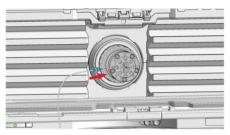
**4** Push the valve head until it snaps in and stays in the rear position.
