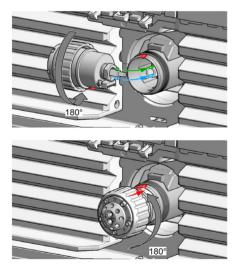
**2** When the outer pin is locked into the groove, manually screw the nut onto the valve head.
