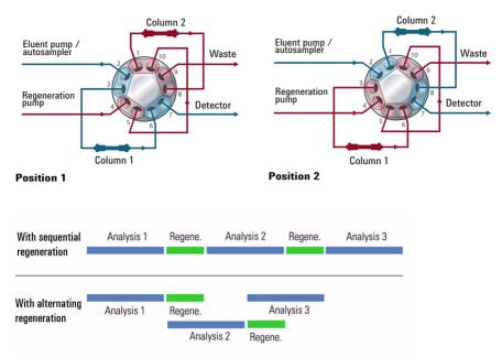
Figure 1 Alternate Column Regeneration (Time Scheme)
