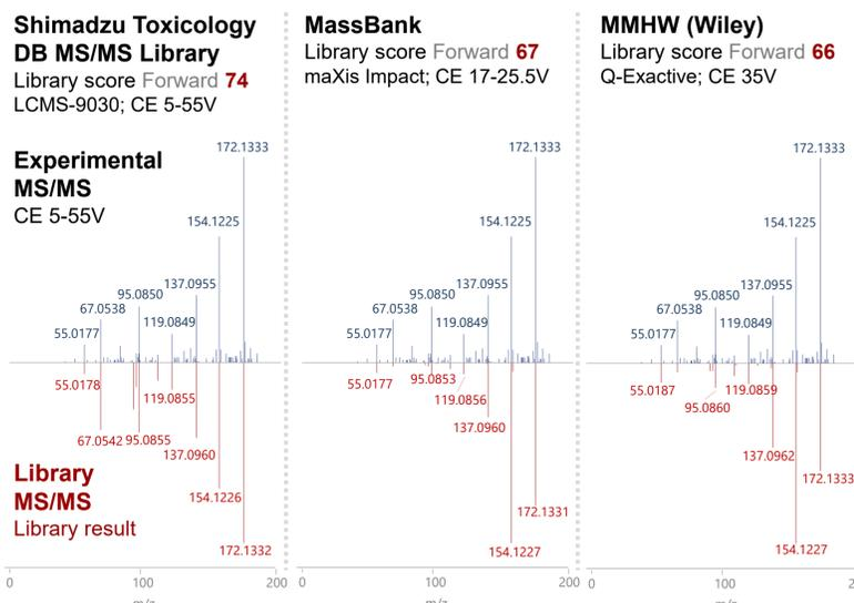
**Figure 2.** Library results for gabapentin (prescribed as an antidepressant, anticonvulsant and treatment for neuropathic pain; C<sub>9</sub>H<sub>17</sub>NO<sub>2</sub>, precursor m/z 172.1332) using multiple data repositories with similar library matches.
